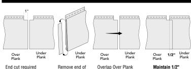
End cut required on Under Plank for proper overlap.
