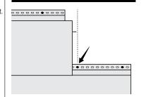
Place a fastener on lower course in nail slot closest to plank overlap. IMPORTANT: See full installation instructions for further details.
